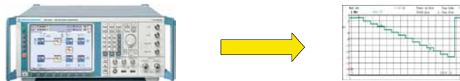
The R&S SMU200A changes the code channel output power on the basis of the TPC field
